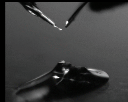
The scanning probe (left) and the microwave antenna (right) approaching the sample (in the lower part of the image) to start the measurement. Image taken with the ProteusQ side view camera.
