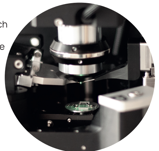
Probe and near-field antenna, with sample retracted
