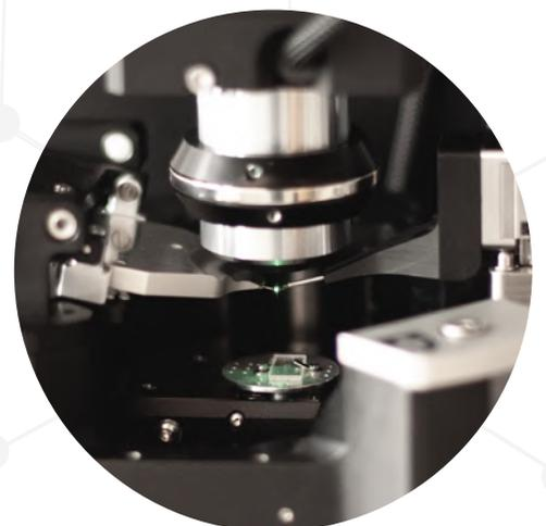
Probe and near-field antenna, with sample retracted
